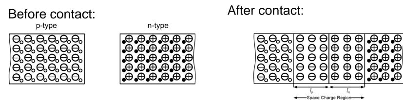
Electrons diffuse into the p-type semiconductor, and holes into the n-type semiconductor. The positively and negatively charged donor and acceptor ions in the *space charge region (SCR)* build up an electric field that counteracts diffusion.
